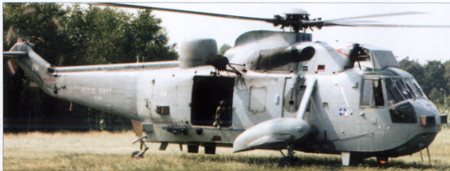
Bottom - note inclination of the blades of the six-blade anti-torque rotor and stabilizer geometry.
