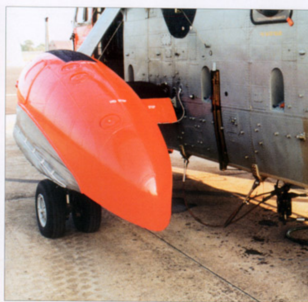
Details of the float nacelles with the main landing gear, bottom centre - a tail wheel.
