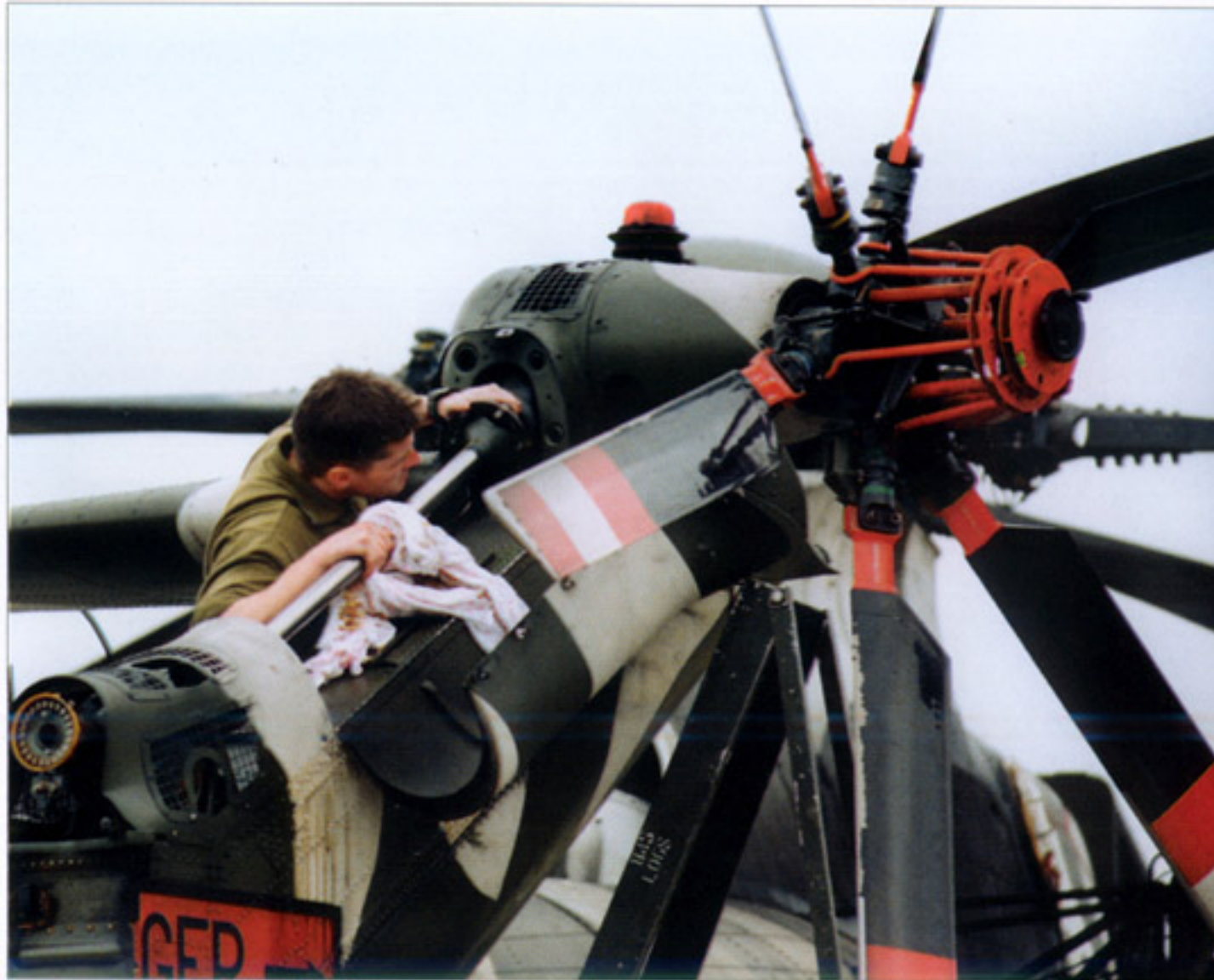
Top and bottom - details of the head of the anti-torque rotor, right - folding mechanism of the tail.
