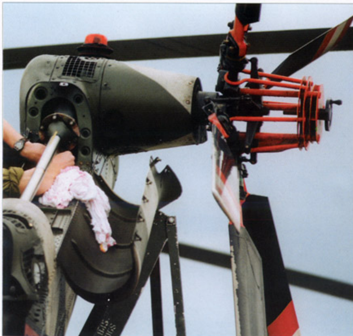
Top and bottom - details of the head of the anti-torque rotor, right - folding mechanism of the tail.
