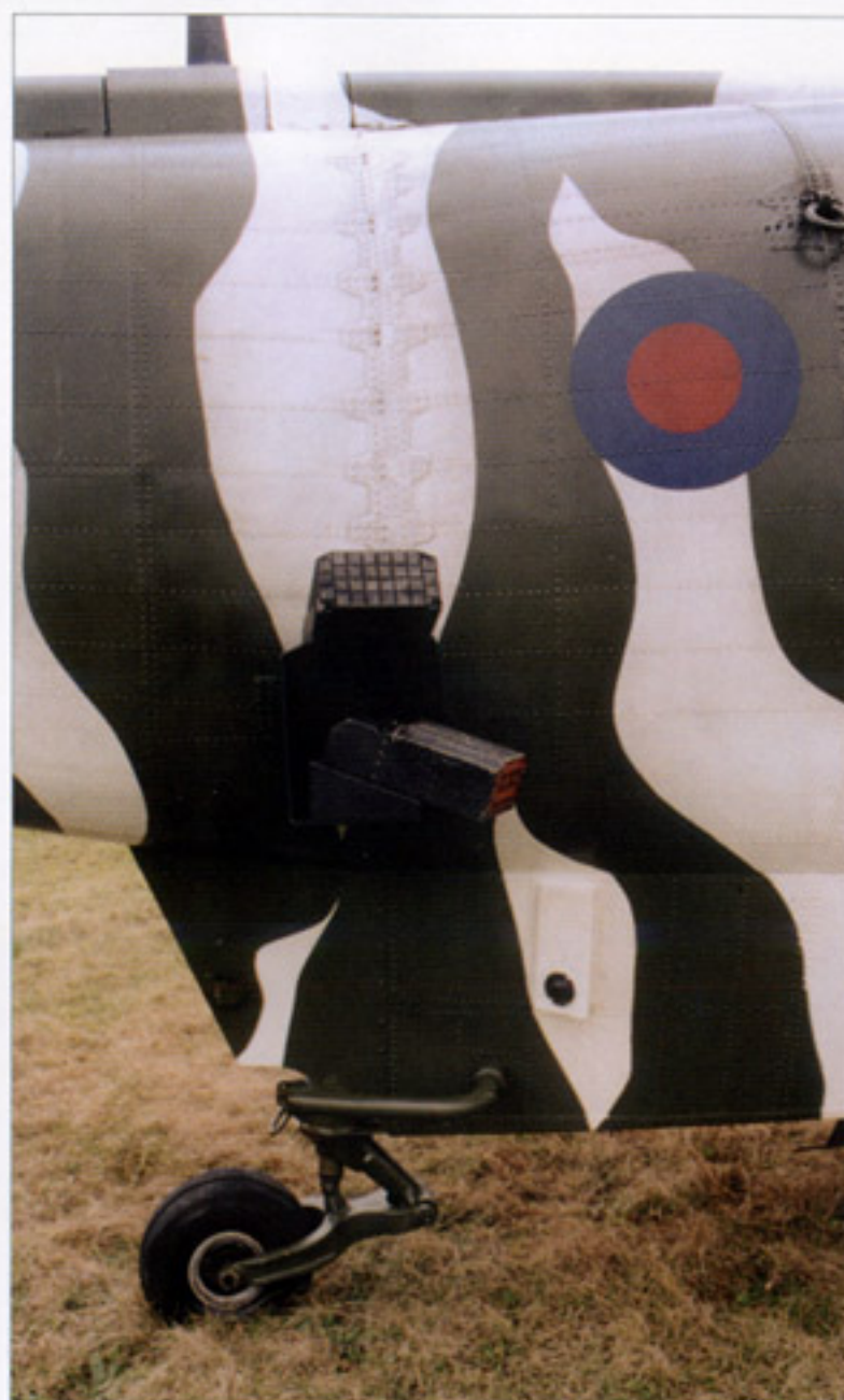
Top - a HC.Mk.4 on an improvised static stand in Bosnia, bottom - details of anti-rocket defence of the machine.
