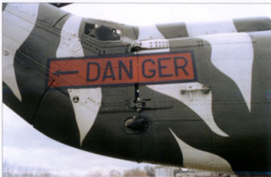
Field maintenance just after landing, Bosnia. Details of the locking device of the folding tail.
