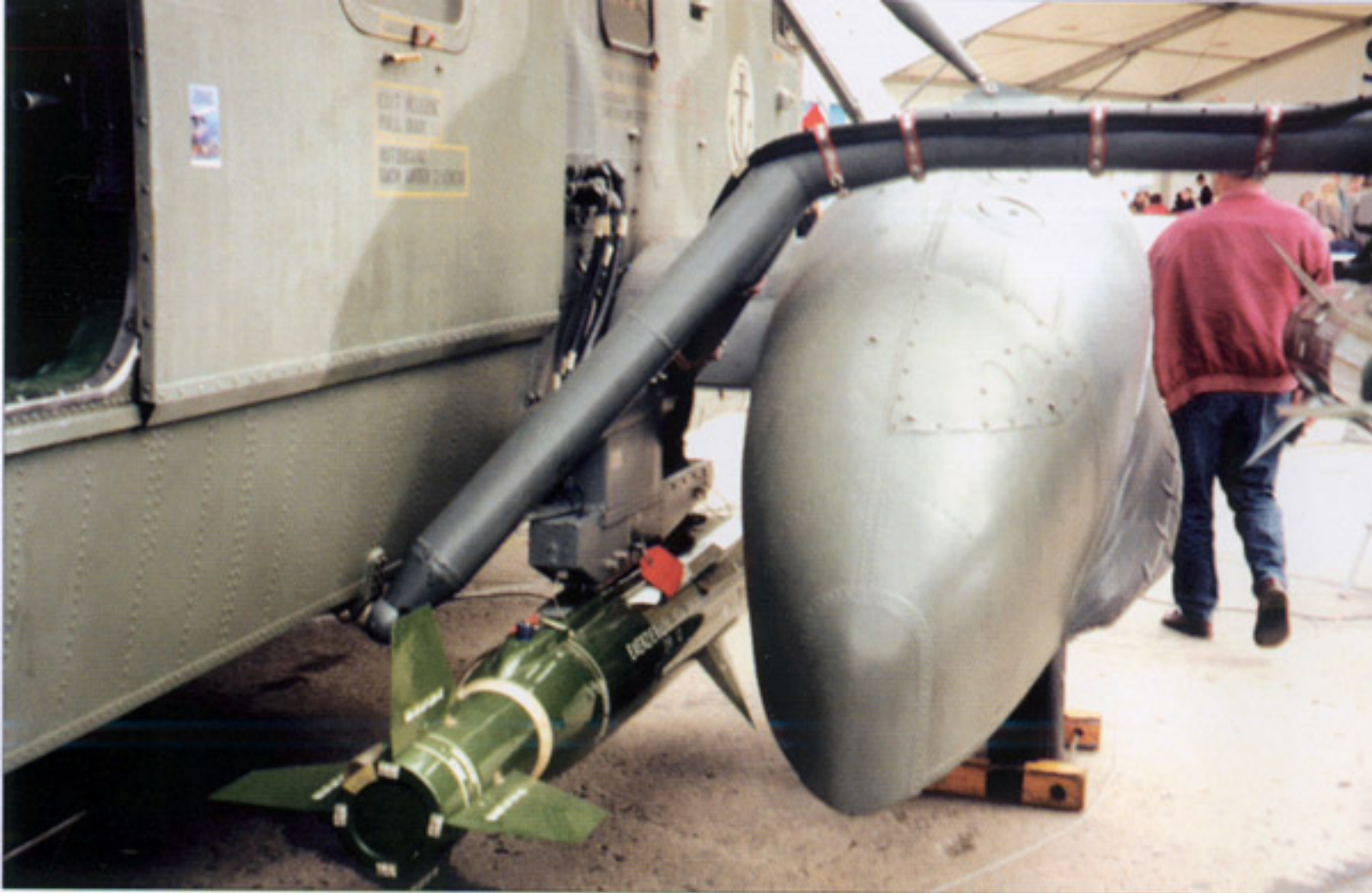
Detail of the place of work of the weapon systems operator, passage in the fuselage and details of the Sea Skua rockets attachment.
