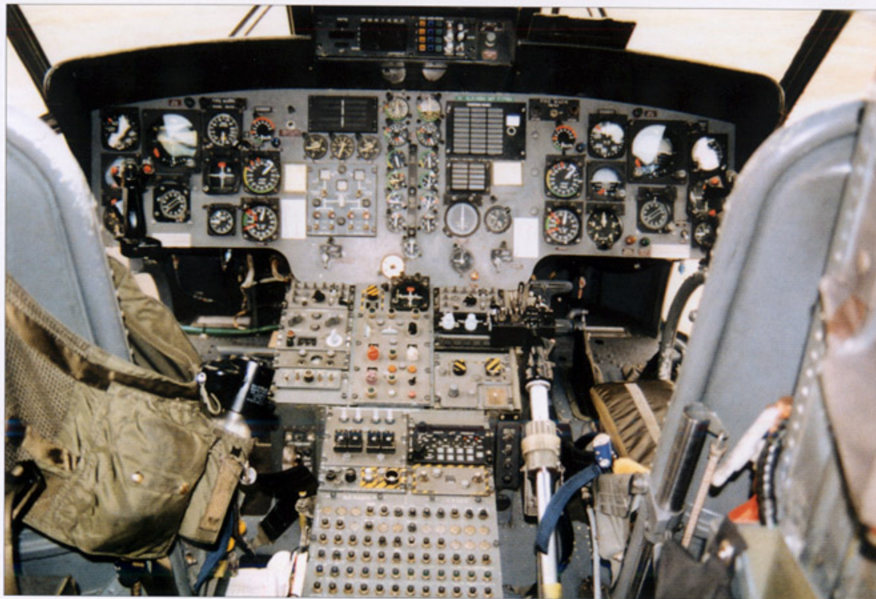
Top - central overhead panel, left - various variants of instrument panels, bottom - panel between the pilot's seats.
