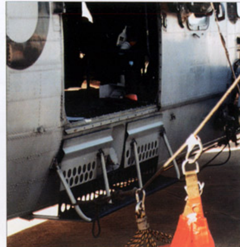
Detail of a foot-hold below the threshold of the cargo compartment door. Detail of the main rotor head and engine.
